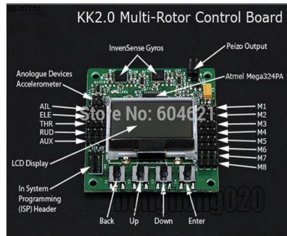
Figure 3 KK 2.0 Multi-Rotor Control Board
