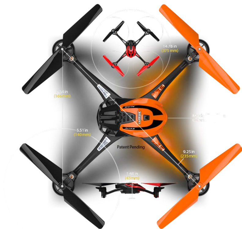
Figure 6.1B: Traxxas 6608 Quadcopter and its dimensions.
