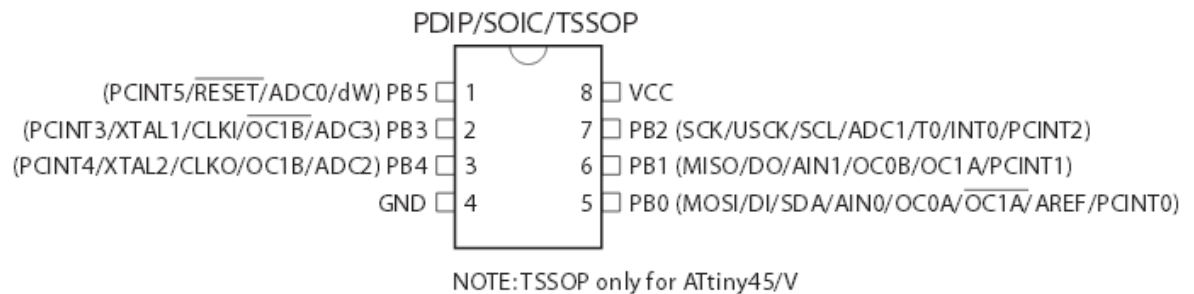
Fig 5.3.1 (1) ATtiny pin diagram (Pending approval from Atmel)
