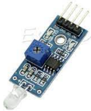
Figure 10 - LM393 Light Sensor
