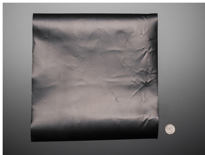
Figure 17: Pressure-Sensitive Conductive Sheet (Velostat/Linqstat)
