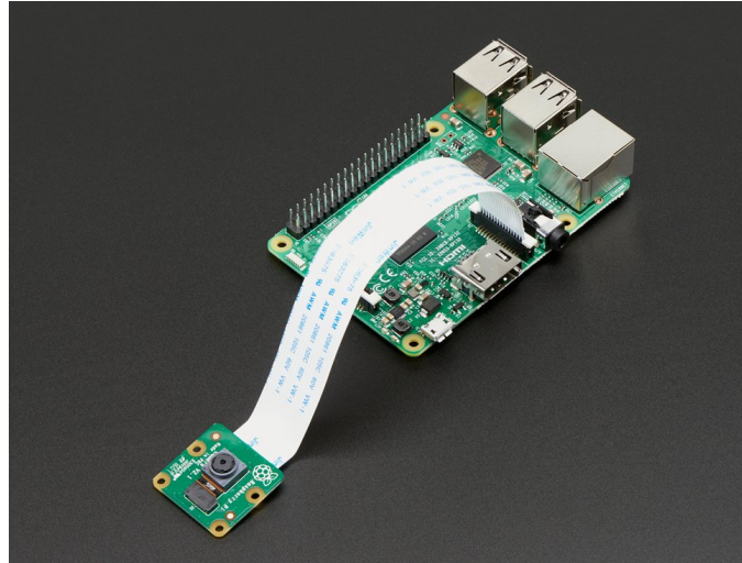
Figure 25: Raspberry Pi camera hooked up to the microcontroller
