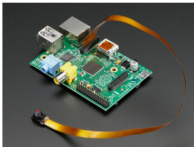
Figure 26: Small spy camera shown hooked up to a Raspberry Pi
