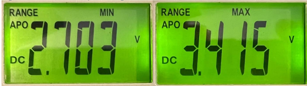
Figure 4.2.2.7 – DC Output Voltage of Ultrasonic Anemometer
