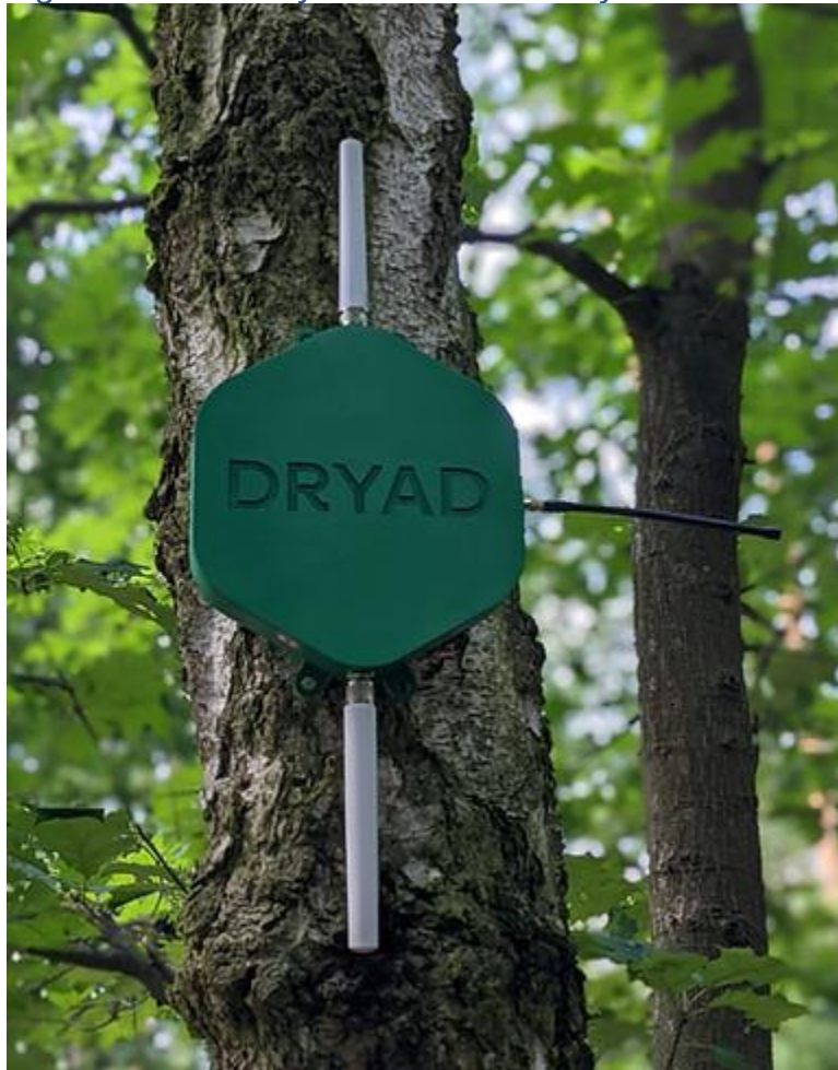
Figure 3.1.1.4 – Dryad Border Gateway
