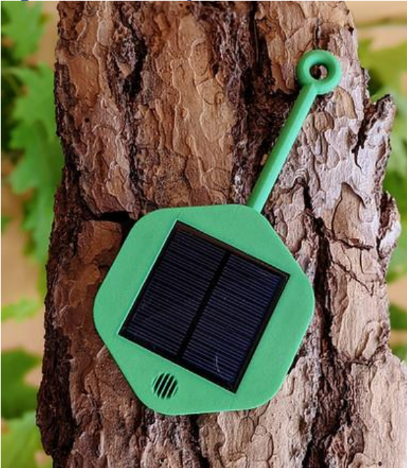
Figure 3.1.1.3 – Dryad Silvanet Wildlife Sensor
