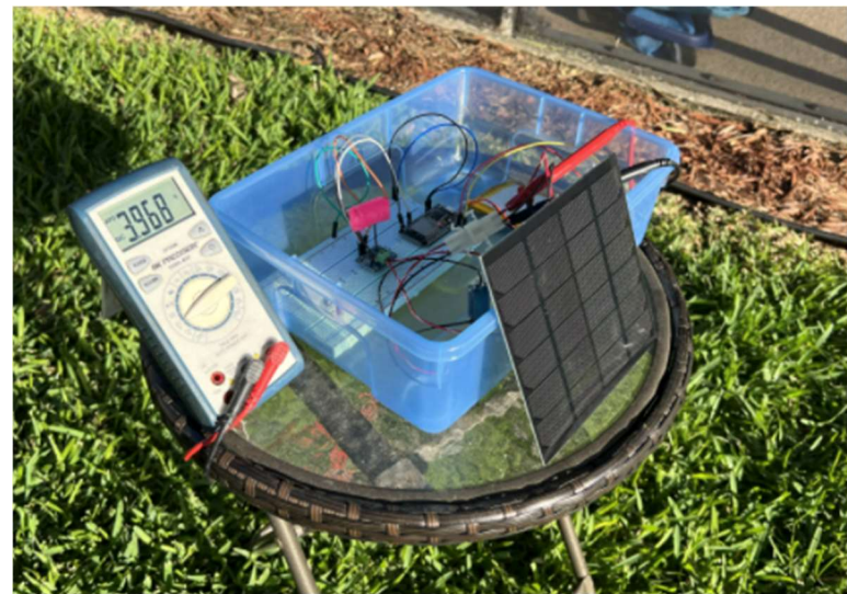
Fig. 2. Solar power system testing apparatus
