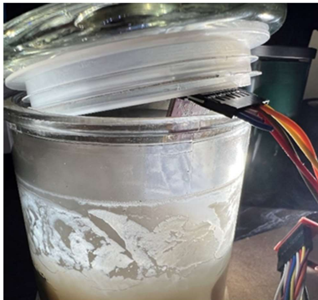
Fig. 4. Testing of CCS811 CO 2 and TVOC sensor
