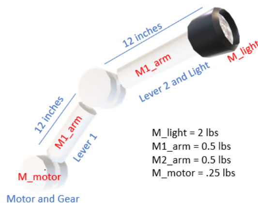
Figure 37: ArticuLight Model for Calculating Torque
