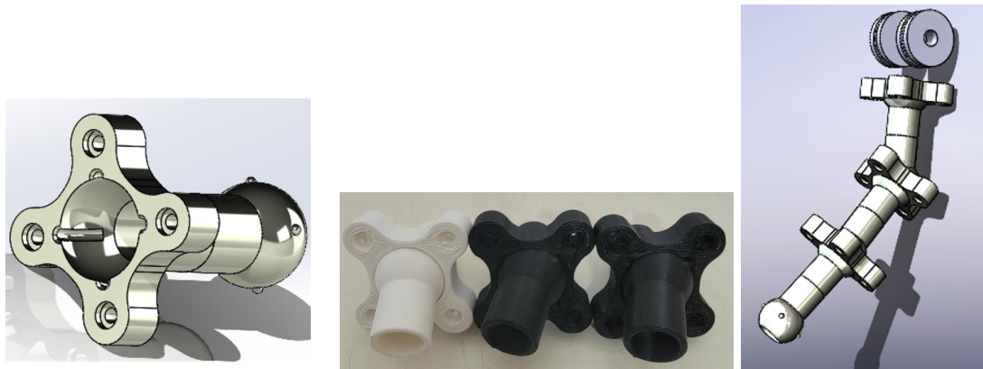
Figure 28: Prototype 4 3D Model, Printed Prototypes 2,3, and 4, and Assembled 3D Model
