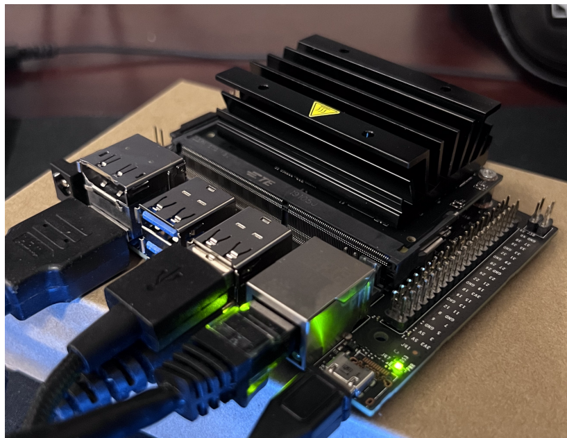
Figure 42: Jetson Nano In Development Stage for Component Testing
