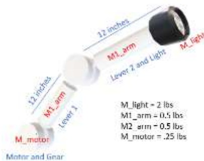
Figure 39: ArticuLight Model for Calculating Torque
