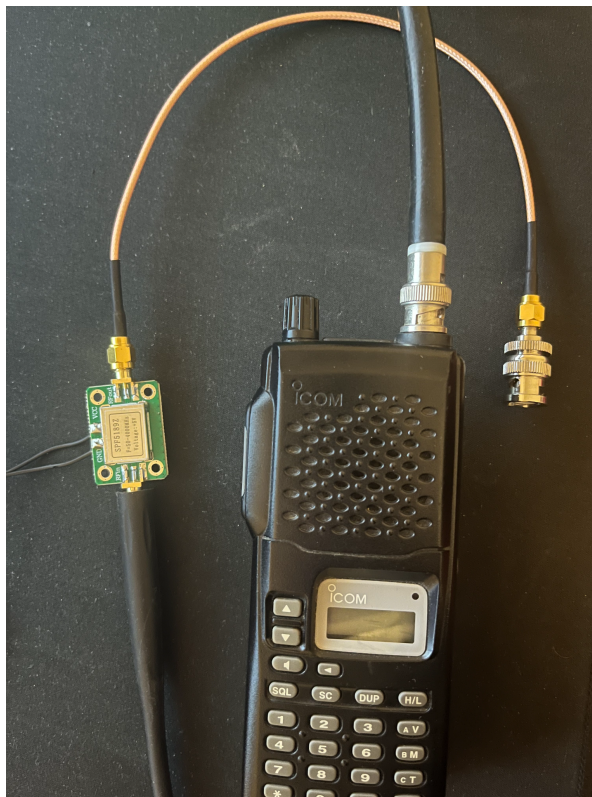
Figure 77. SMA to BNC connection
