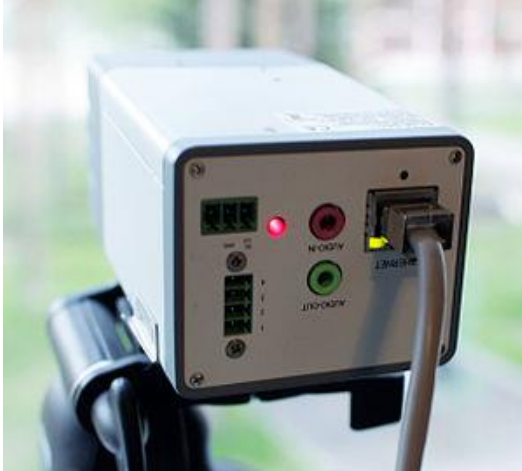
Figure 1: IP camera powered by over ethernet. CC0 1.0 Universal (CC0 1.0). Public Domain Dedication.
