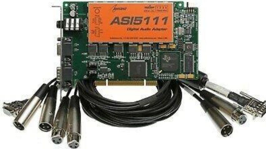
Figure 9: PCI Microphone connector card that directly supports XLR. Reproduced under CC BY-NC.
