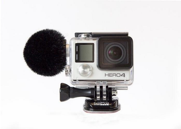
Figure 6: GoPro with external microphone and wind muff. Reproduced under CC BY-NC.
