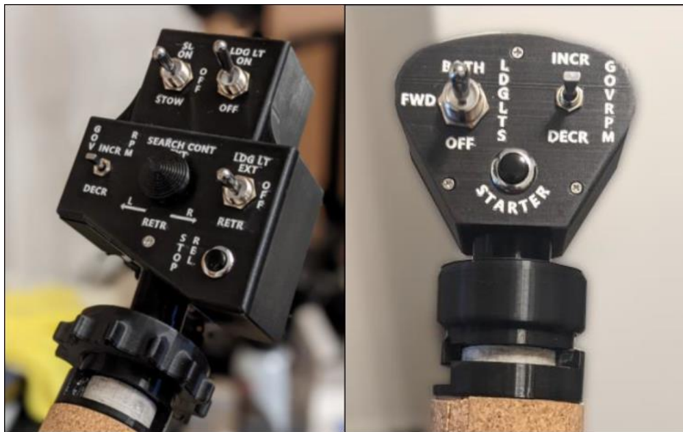
Figure 39 – Interchangeable UH-1 Huey and Bell 206 Heads
