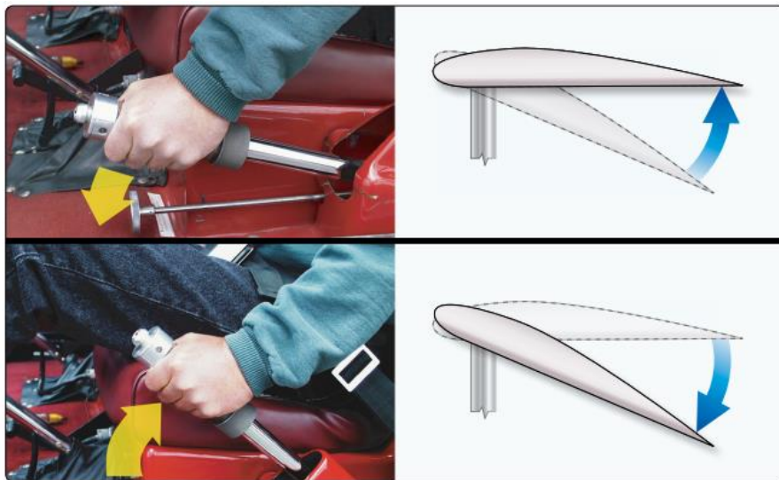
Figure 3 - Effect of Collective Lever Movement on Rotor Blade Pitch Angle
