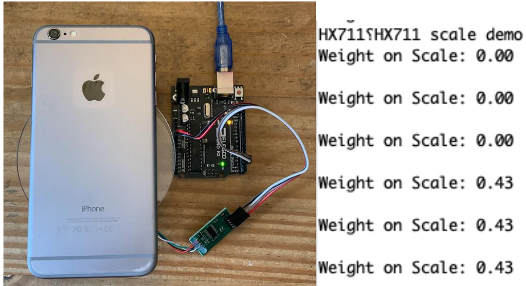
Figure 101: Load Cell Test #1 Setup and Results
