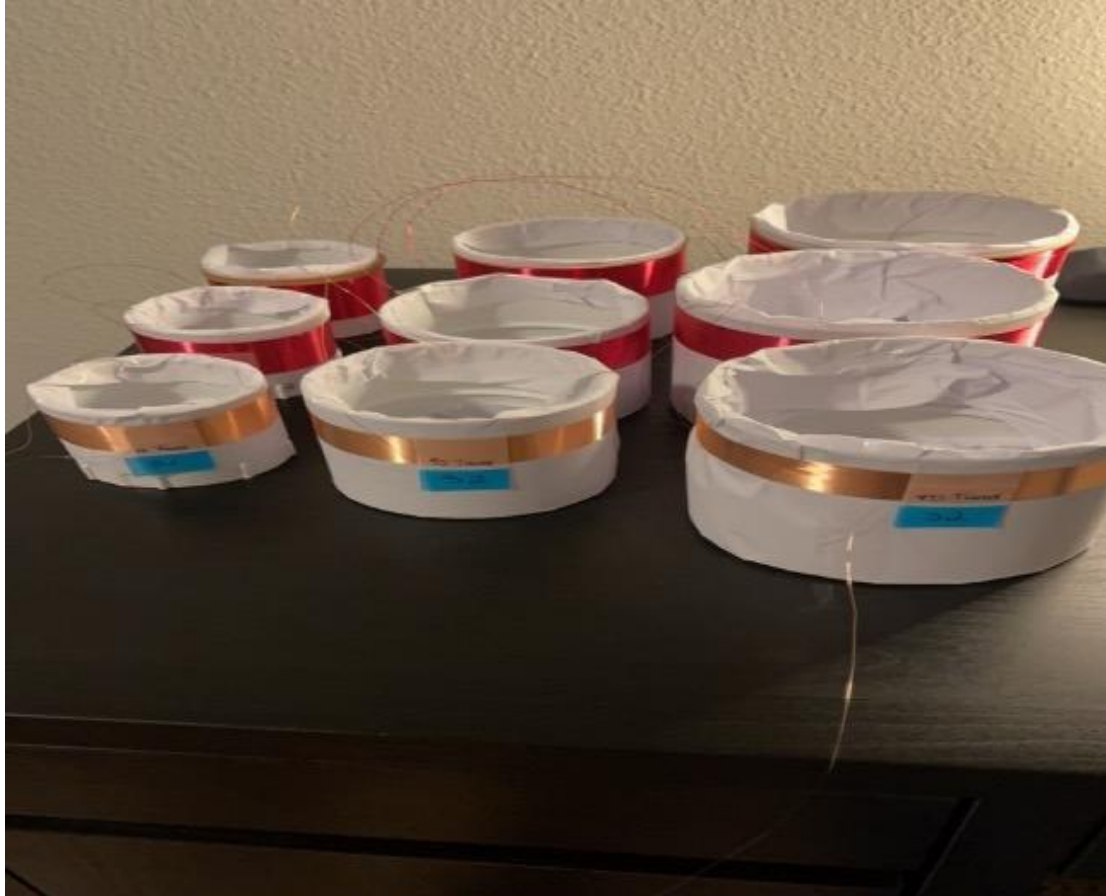
Figure 71: PVC wired with enameled copper
