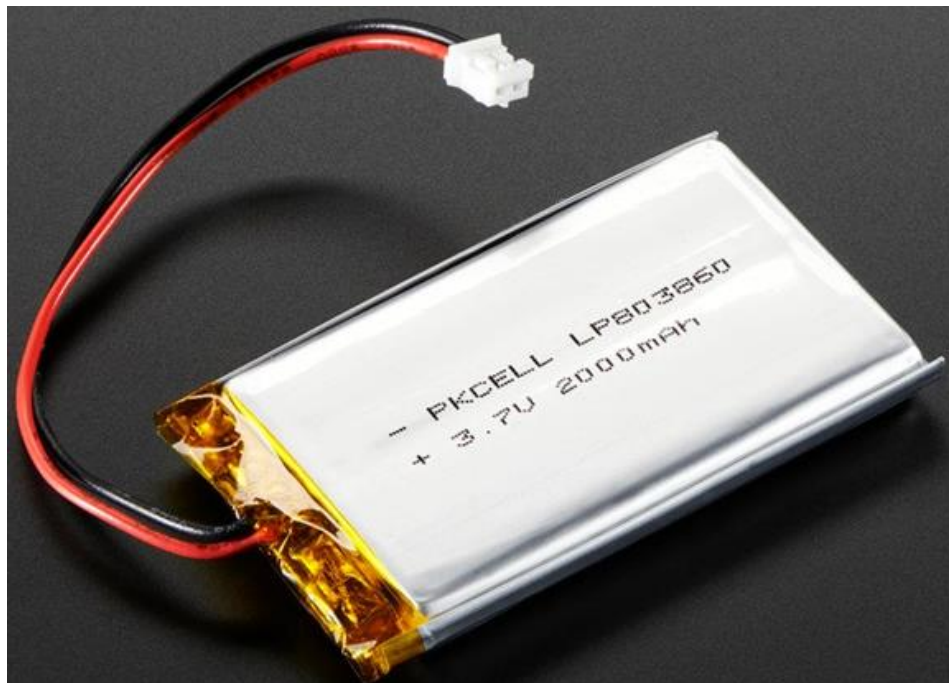
Figure 23: Lithium-ion battery (probable power source)
