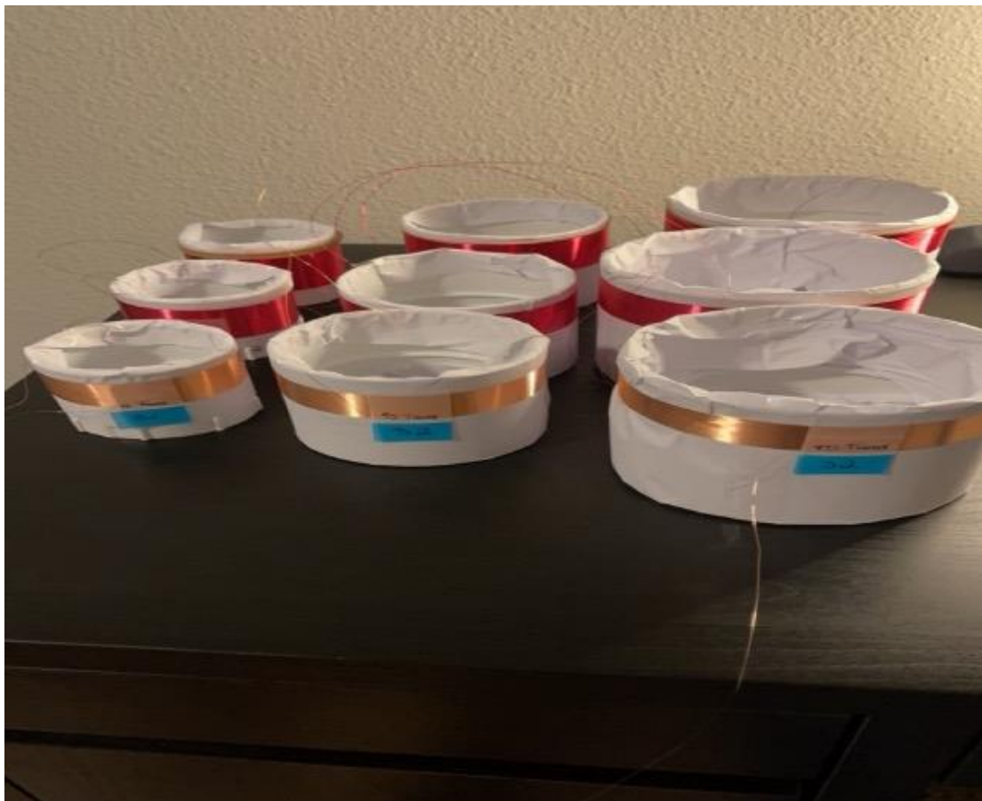
Figure 71: PVC wired with enameled copper
