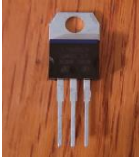
Figure 21: Voltage regulator L7805CV
