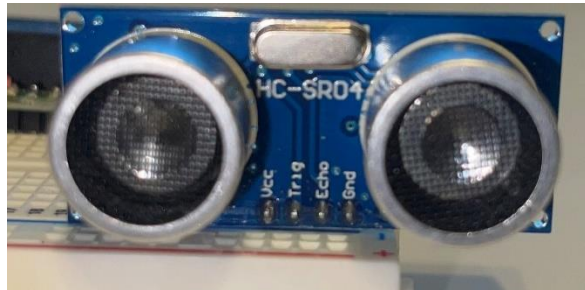
Figure 15: HC-SR04 Sensor on Breadboard Showing the Pins. The figure shows the Ultrasonic Sensor of our choice.
