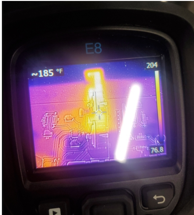
Figure 103: FLIR Reading for PMOS
