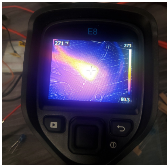
Figure 102: FLIR Reading for Schottky Diode
