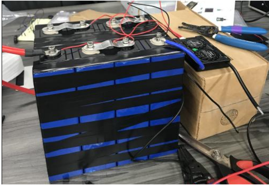
Figure 105: Battery Cells Assembled with BMS
