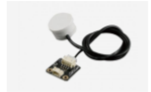
Figure 5-11: Water Level Sensor
