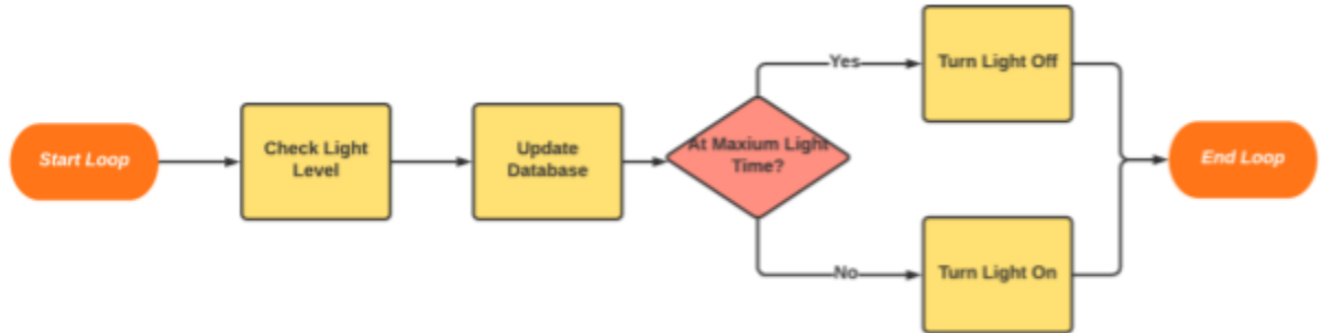
Figure 6-20: Light Sensor Monitoring
