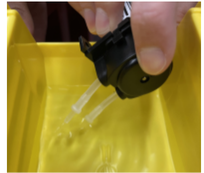
Figure 5-13: pH Balancing Pump
