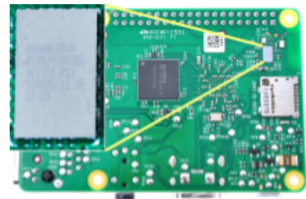
Figure 6-29: Raspberry Pi WiFi card
