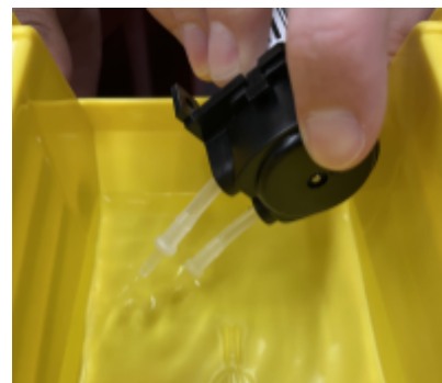
Figure 5-11: pH Balancing Pump
