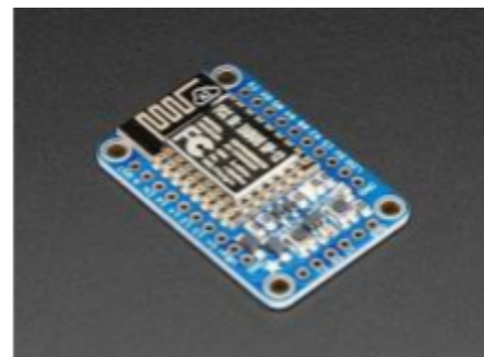
Figure 5-3: Adafruit HUZAZH WiFi Module
