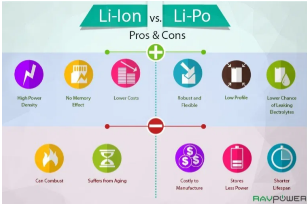
Figure 5-2: Li-Ion vs. LiPo[17]
