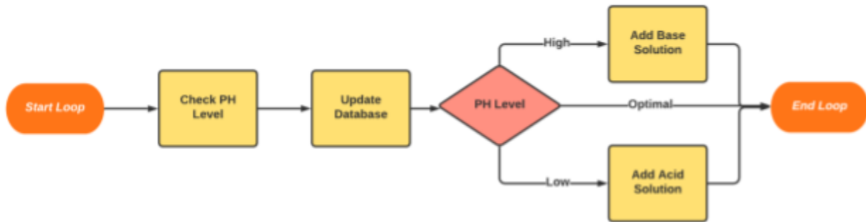
Figure 6-24: pH Sensor Monitoring
