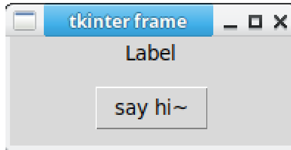
Figure 32. A simple example of a frame in Tkinter with a label and a text of “say hi~” One can imagine how you can expand upon this simple concept.
