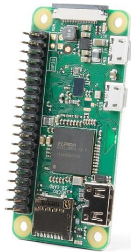
Figure 10 (Used with the permission of Helen Lynn). The Raspberry Pi Zero is an extension of the Pi Zero family that launched in early 2017. It has all the
