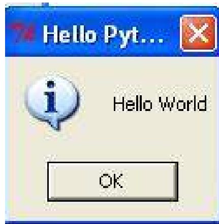
Figure 33. An example of a button object being used in a frame of a root window. One can distinguish between the three objects by noting that the root is the window itself, the frame is the beige color, and the button is the rectangle with the text “OK”.
