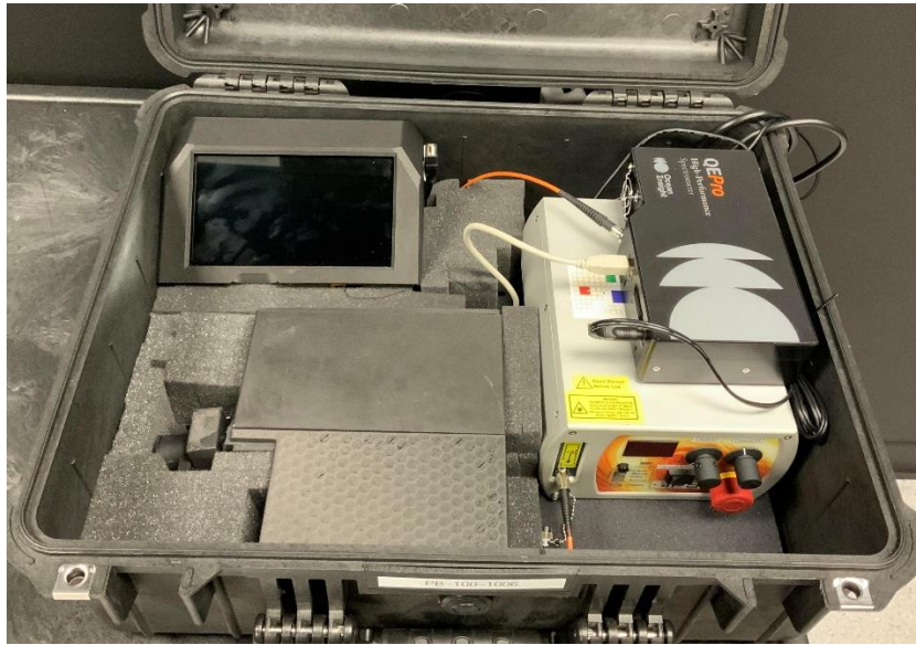
Figure 40. Optical box design in pelican case
