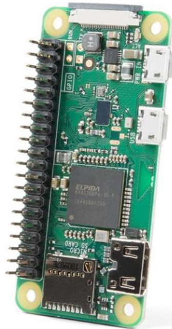
Figure 10 (Used with the permission of Helen Lynn). The Raspberry Pi Zero is an extension of the Pi Zero family that launched in early 2017. It has all the functionality of the original Pi Zero with added connectivity and more powerful computing power. It offers Linux capabilities as well as the NOOBS
