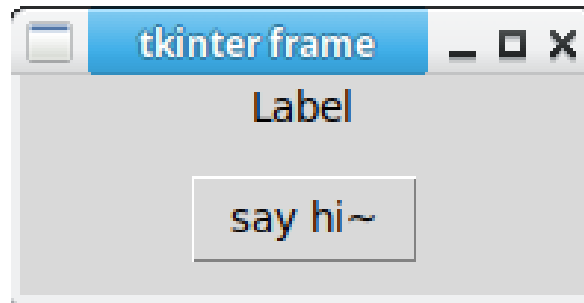
Figure 26. A simple example of a frame in Tkinter with a label and a text of “say hi~” One can imagine how you can expand upon this simple concept.
