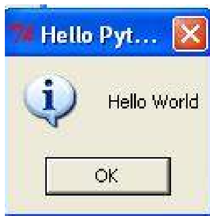
Figure 27. An example of a button object being used in a frame of a root window. One can distinguish between the three objects by noting that the root is the window itself, the frame is the beige color, and the button is the rectangle with the text “OK”.
