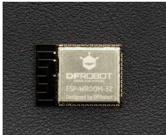
Figure 4. ESP32 (ESP WROOM 32) WiFi + Bluetooth (Courtesy of Digi Key) First choice for project
