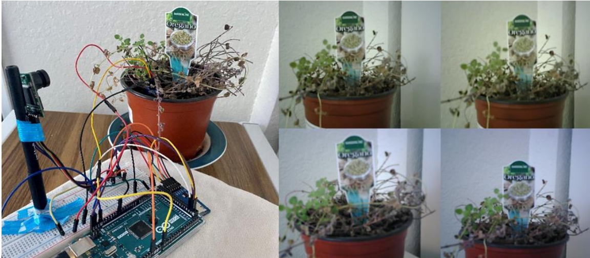
Figure 30: Test Setup for OV2640 Camera Module and Pictures in Different Lighting and Position
