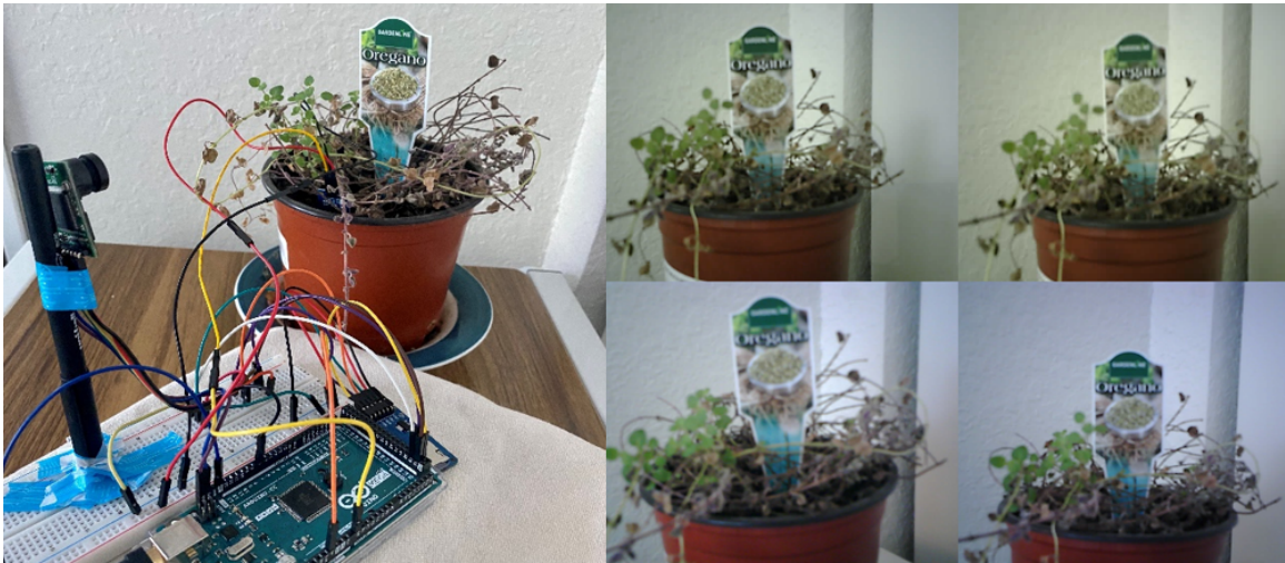
Figure 27: Test Setup for OV2640 Camera Module and Pictures in Different Lighting and Position
