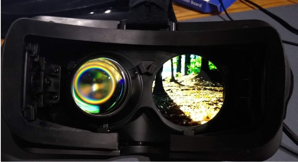
Figure 32: The Oculus Rift configured as a secondary monitor is shown with one lens removed, to demonstrate barrel distortion
