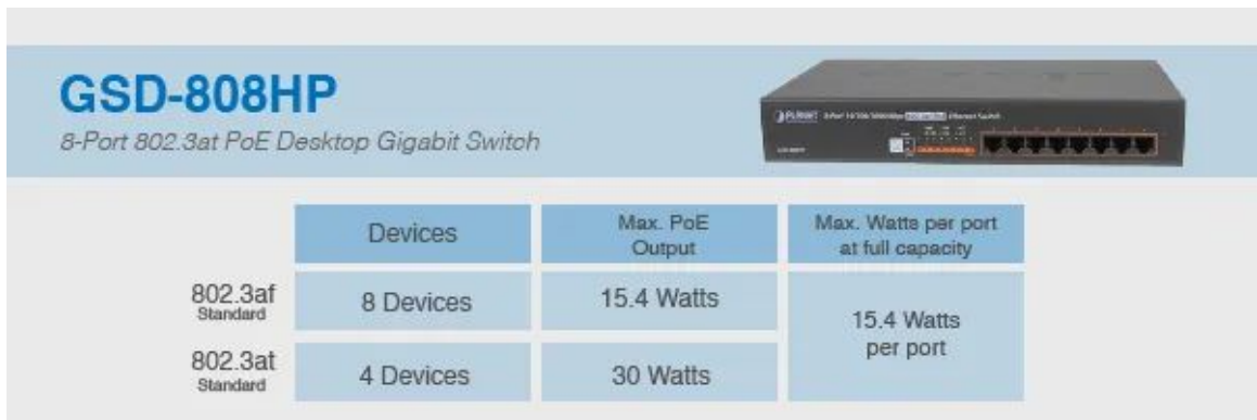
Figure 23: Network switch and standards for PoE output Reprinted with permission, from [20]
