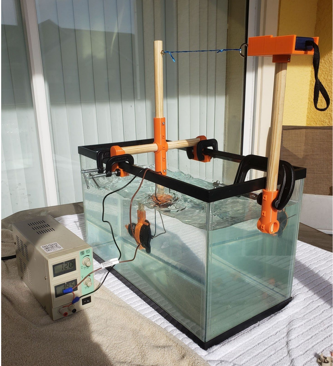
Figure 49: Motor Test Bench
