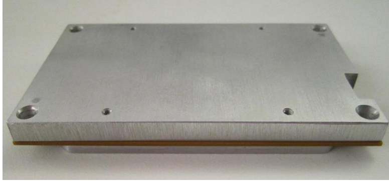
Figure 53. Image above shows the passive cooling Thermal Transfer Plate that comes with the Nvidia TX2.
