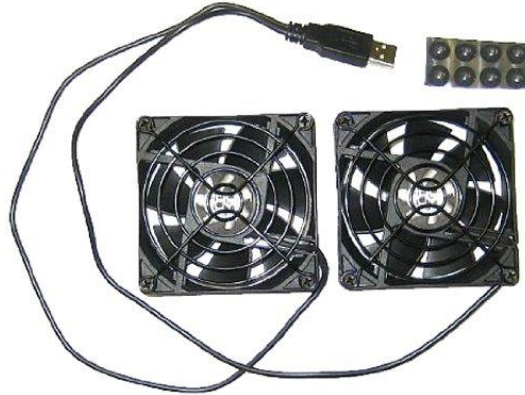
Figure 55. Image above shows the fans that will be used as an additional cooling mechanism for Sean.
