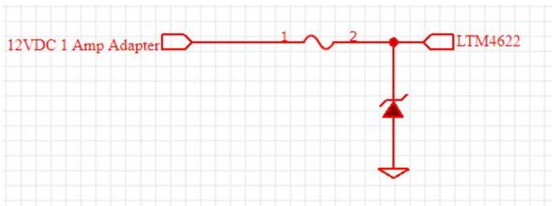
Figure 5-16: Overcurrent and Overvoltage Protection Design
