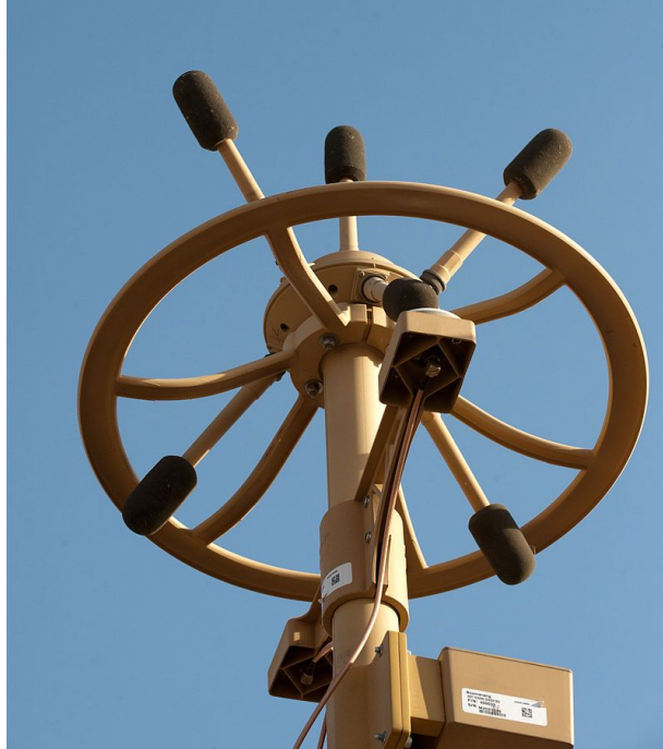
Figure 4-1: Boomerang III microphone cluster. Open Government License. Obtained from wikipedia.
