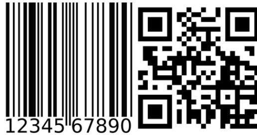
Figure 26 - 1D (left) and 2D (right) Barcodes (Permission to reproduce submitted)
