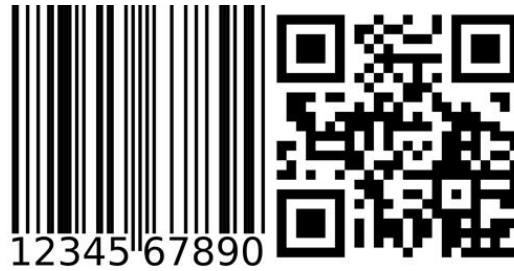
Figure 27 - 1D (left) and 2D (right) Barcodes (Permission to reproduce submitted)
