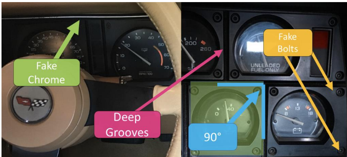
Figure 72 - shows minimalism and hard edges in 1982' Corvette interior that was a result of material/manufacturing limitations of the era. Created by Mikey Garrity
