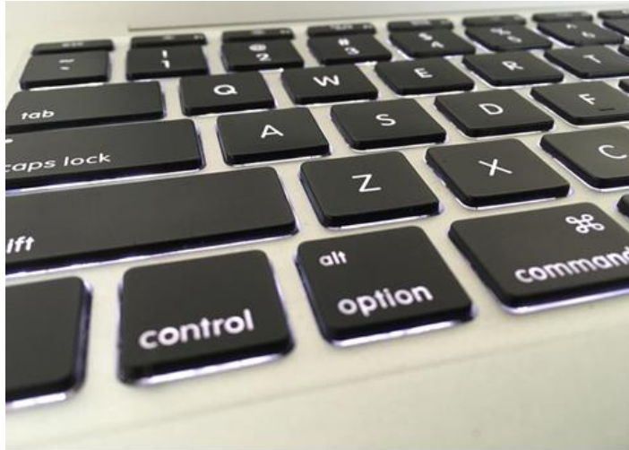
Figure 25 - is an image of Apple's MacBook Air portable computer demonstrating the auto brightness of the keys based on built in Ambient Light Sensor. Created by Mikey Garrity.
