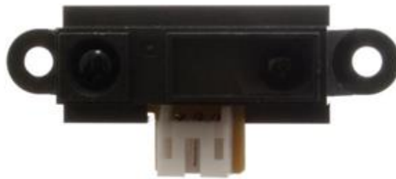
Figure 23 - Shows an image of the Infrared sensor designed by Sharp that is similar to what we implemented in our table. Courtesy of Oomlout, Creative Commons 2.0
