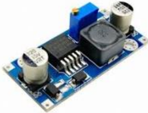
Figure 15 LM2595s Step down Buck Converter.
