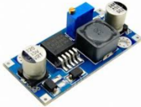
Figure 15 LM2595s Step down Buck Converter.
