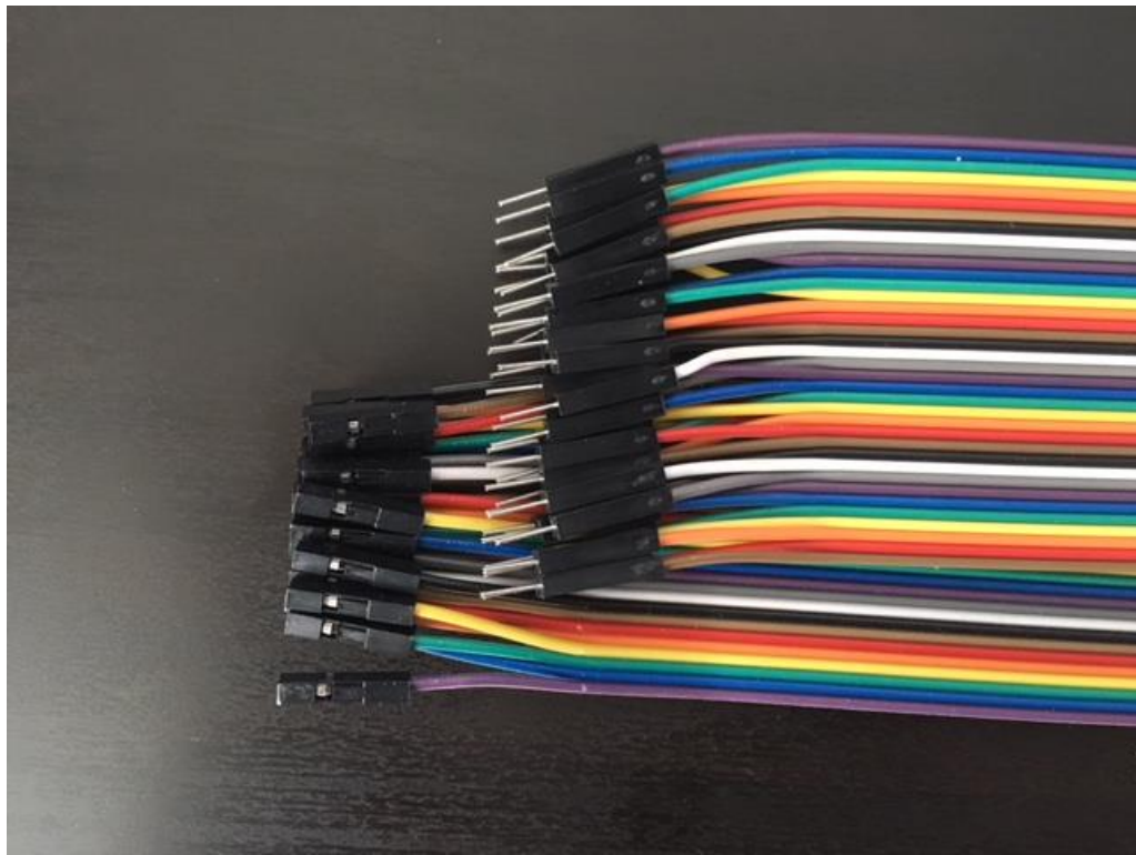
Figure 25: Pre-terminated cabling used for prototyping
