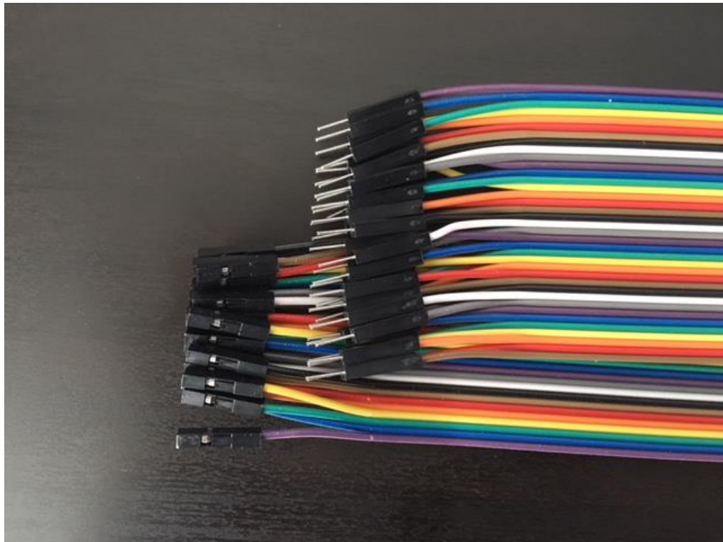
Figure 25: Pre-terminated cabling used for prototyping
