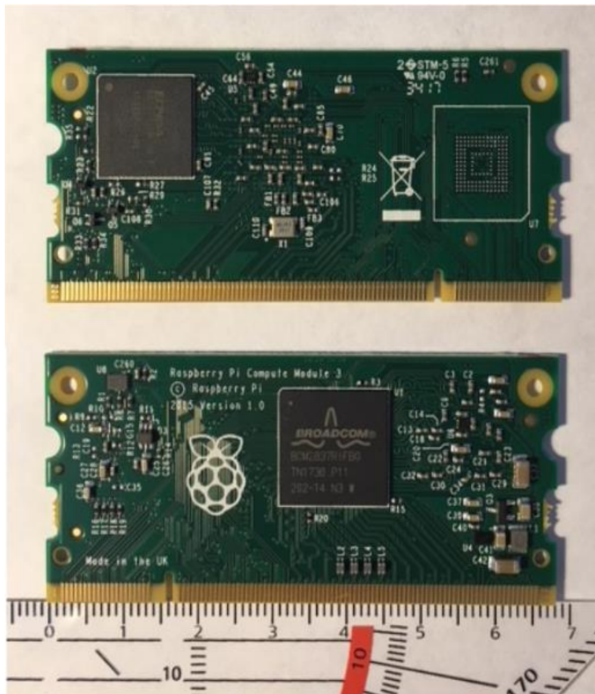
Figure 11: Raspberry Pi Compute Module 3L back and front with cm measure for scale
