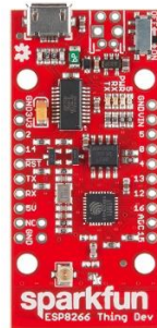
Figure 13: Sparkfun ESP8266 Thing Dev Board – Image credits to SparkfunTM ElectronicsSparkfun ESP8266 WiFi Module
