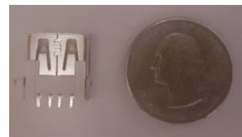
Fig. 9. The USB type A socket to be used for connecting the microphone and speakers along with troubleshooting if required.
