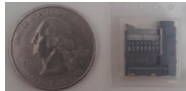
Fig. 8. The microSD card socket used to store the device's operating system.
