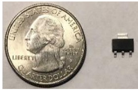
Fig. 11. The LM317MBSTT3 linear dropout voltage regulator used to regulate certain voltages required by the device's components.
