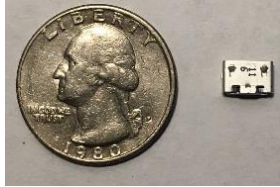
Fig. 10. The microUSB port that is used to accept an input power source. It is responsible for powering the PCB.
