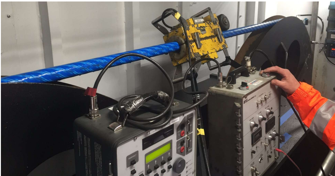
Figure 1: Worker pulling a steel wire rope through a magnetic flux leakage testing device.
