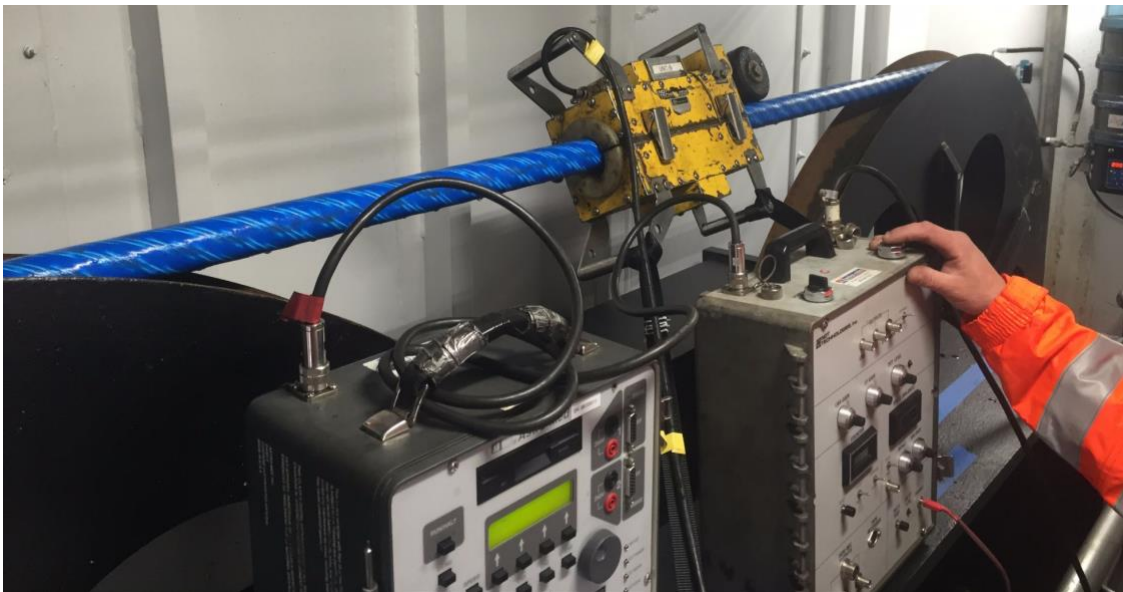
Figure 1: Worker pulling a steel wire rope through a magnetic flux leakage testing device. (Permission with inter mtn pending)
