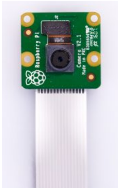
Figure 17: Raspberry Pi 3 on Board Camera Permission to use granted by Helen Lynn, Raspberry Pi foundation.
