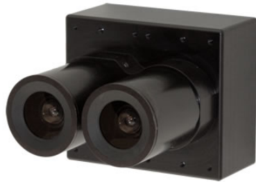
Figure 5: Example of a Simple Stereo Camera.
