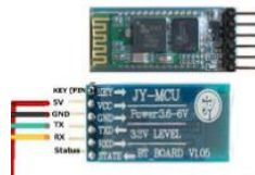
Figure 3.1.12.5 - HC-05 Bluetooth External Module with a Breakout Board [Techbitar]
