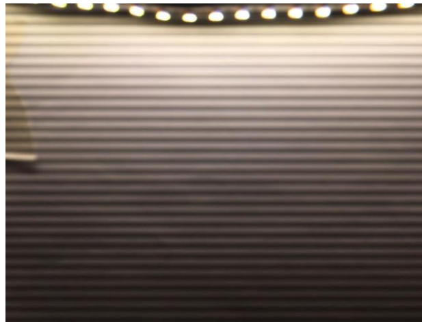
Figure 7.4 - LED PWM Cycle Desync
