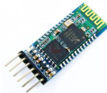
Figure 3.1.12 - HC-05 Bluetooth Module
