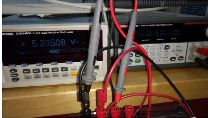
Figure 5.4.1 –Voltage Regulator Output
