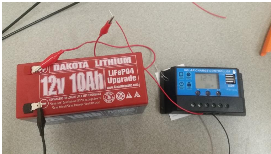
Figure 5.9-1: Battery voltage read by controller
