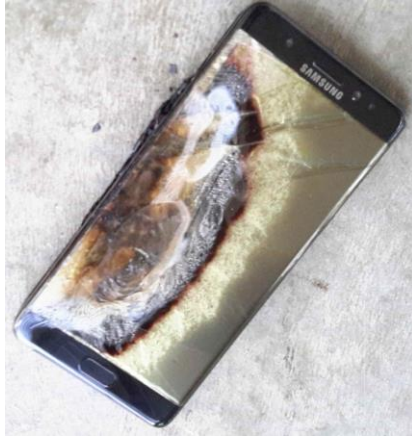
Figure 3.4.4: Example of Faulty Samsung Battery [42]
