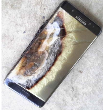
Figure 4.4.5.0: Example of Faulty Samsung Battery [10]
