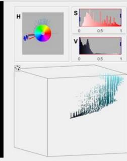
Reflected light can confuse the robot, this additional noise needs to be filtered out with morphological processing in order for the robot to correctly track the correct object.
