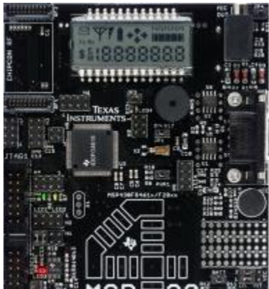
FIGURE 20-MSP430 MCU ON DEVELOPMENT BOARD
