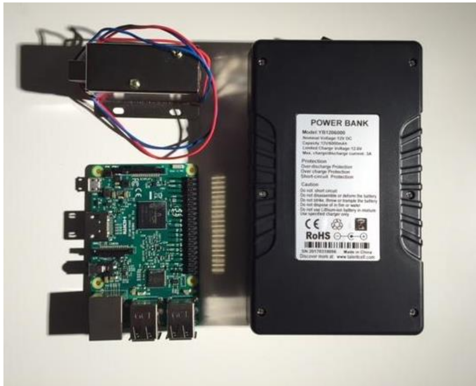
Figure 29 - Door Lock Solenoid, Power Bank, and Raspberry Pi 3
