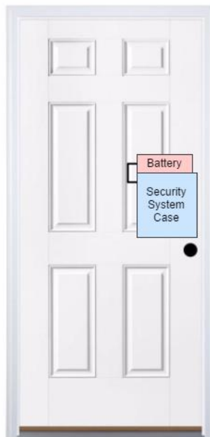
Figure 22 - Outside A1 Security System Mounting
