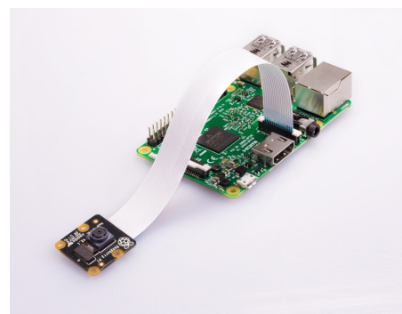
Fig. 2 - Raspberry Pi 3 Interfaced with NoIR Camera
